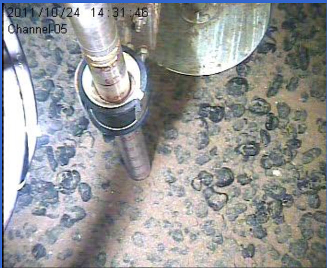
Vane operation on the sea bed
